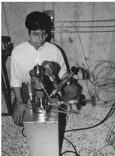
Fig. 14-10 0.5 L stirred autoclave reactor in a high-pressure cell (FH Mannheim, Germany)
