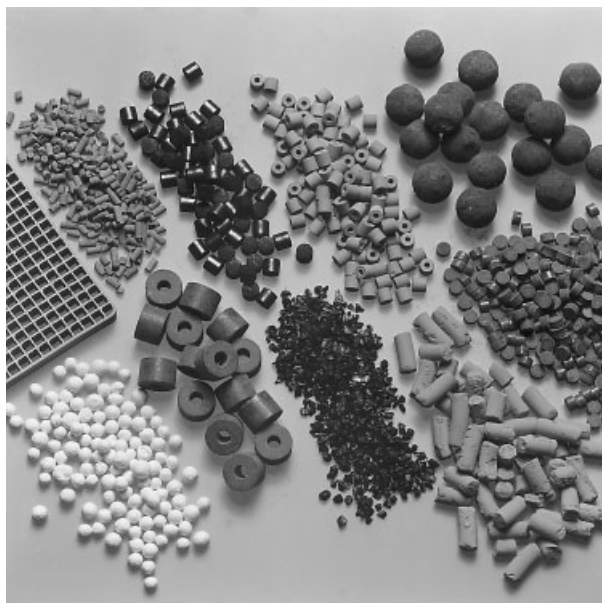
Fig. 6-1 Various shaped catalyst bodies (BASF, Ludwigshafen, Germany)
